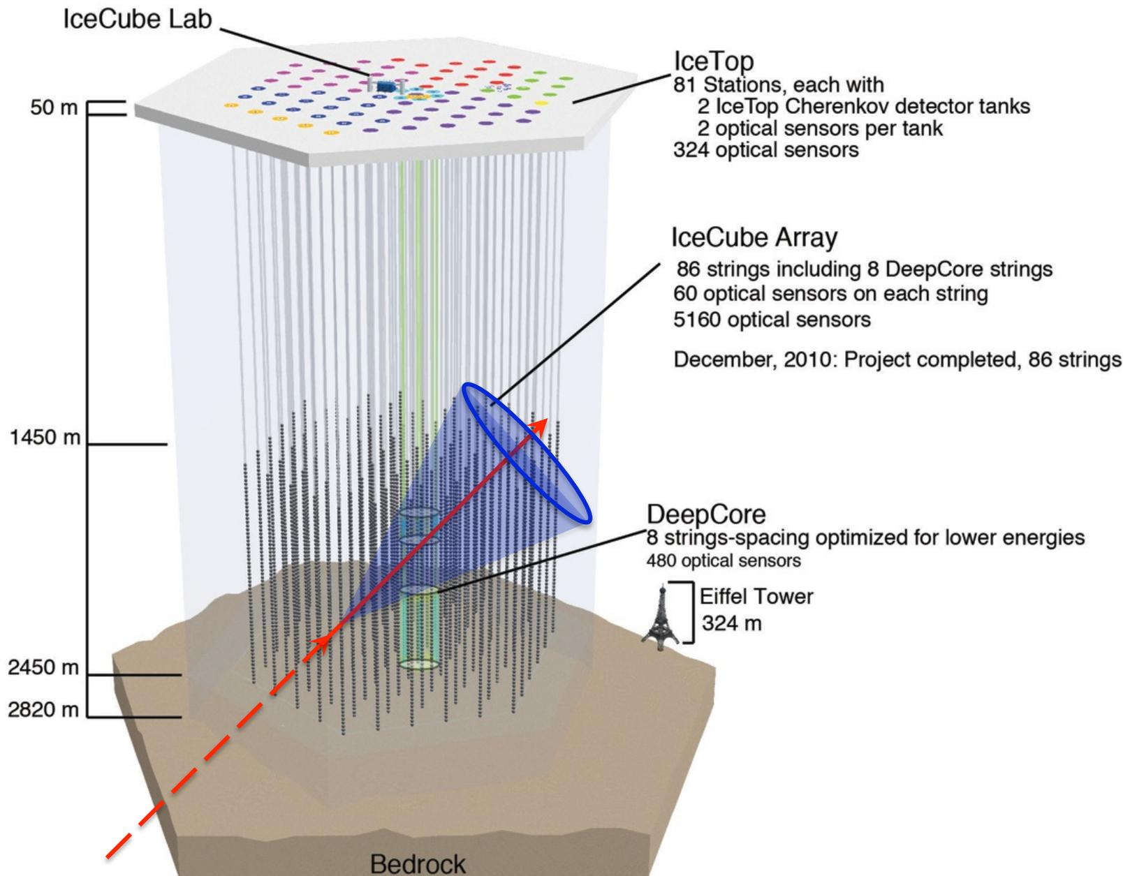
Neutrinos and cosmic rays are detected using Cherenkov emission in ice sheet
